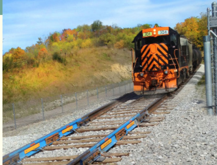
The Avery Weigh-Tronix Weighline is a ballast-mounted checkweigher.
